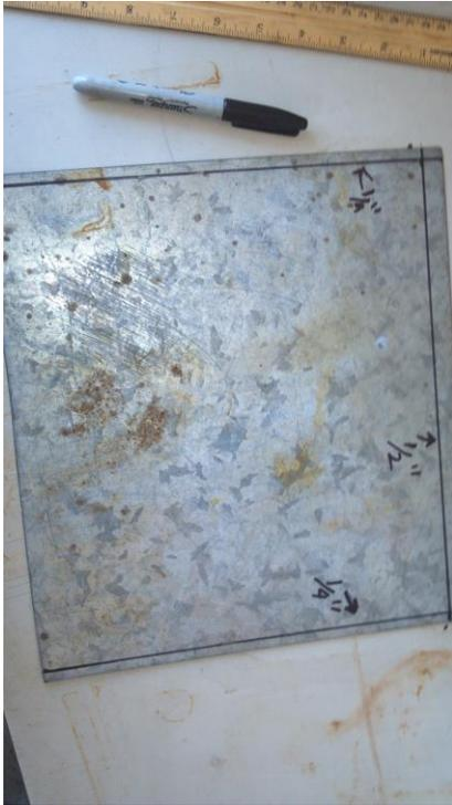
The sheet of metal shows where we bent the two sides and the bottom to snug up against the ice chiller. The best way to bend the sheet is to stick it inside of a vise like the following picture shows.
