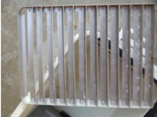
We took aluminum flat stock and bent it at about 130 degree angles and then riveted it to another piece of bent aluminum. Now we know what you are thinking, well maybe we do. That this is way too crazy and I just wanted it to be simpler. Well you can make it simpler. Below we will show you a simpler version.
